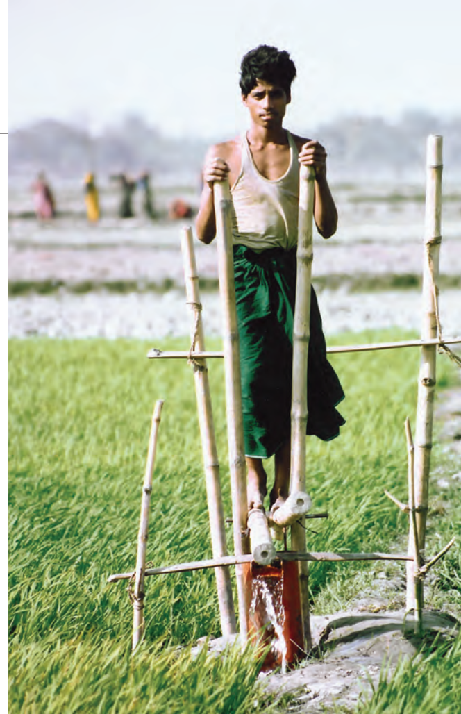
Above: Bamboo treadle pump. Designer: Gunnar Barnes and International Development Enterprises Nepal; manufacturer: small- and medium-sized local workshops, Nepal and Bangladesh, 2006; metal, plastic, bamboo; dimensions: 5’h x 2.5’w x 7’d
